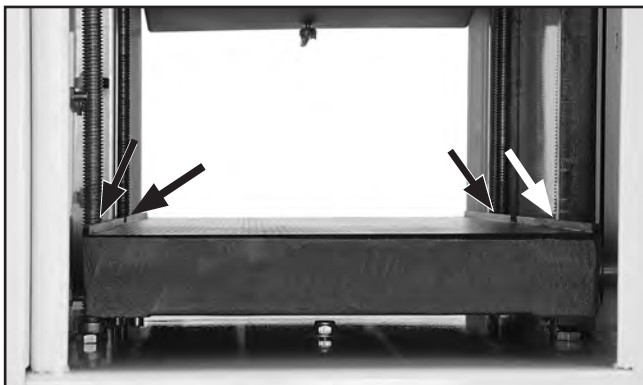
Figure 51. Leadscrew-planer table lubrication locations.
